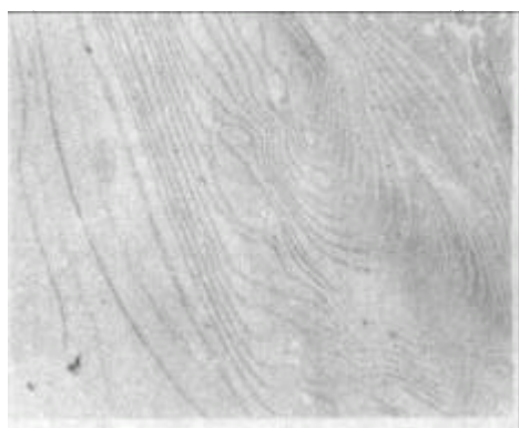
Fig. 7 Morphology of PEO crystallized at 54°C for a period of time beyond 150h
